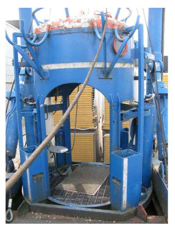
We are pleased to offer for sale direct from Owners this wet-bell, LARS and control cabin. The equipment was originally built by Drass and is offered on an 'as is where is' OR fully refurbished basis.
